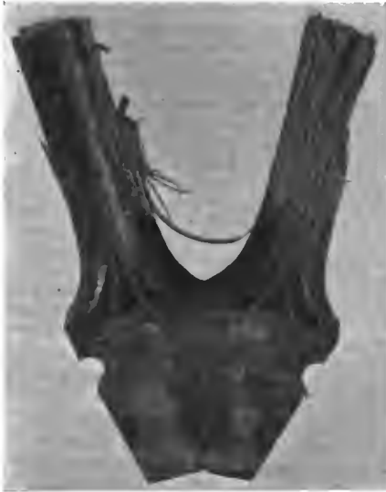
Fig. 29—Depleting part of a broken wheel with more uniform grain and no discoloration whatever
